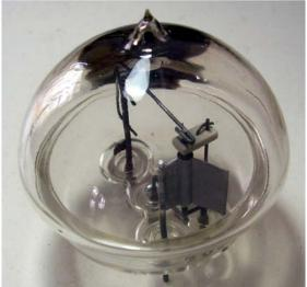
German GEMA designed these tubes to be used in a push-pull oscillator in the Seetakt transmitter, delivering about 1.5 kW at about 375 MHz. Tubes were mounted back-to-back at the ends of the resonating lines, hence the need for specular pinout in the TS1a.
